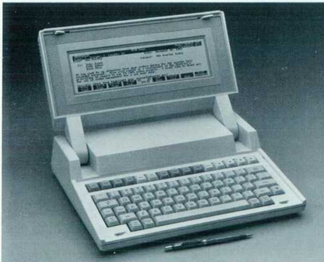
Fig. 1. The Portable (left) comes complete with MS™-DOS 2.11, HP's Personal Applications Manager, MemoMaker, and Terminal Emulation software, and 1-2-3™ from Lotus™. The Portable contains 272K bytes of memory, a 300-baud modem, an RS-232-C/V.24 serial interface, an HP-IL interface, a 16-line-by-80-column liquid-crystal display, lead-acid battery power supply, and a full-size keyboard. The Portable Plus (right) comes complete with MS-DOS 2.11, and HP's Personal Applications Manager, SECURE, HPLink, EDLIN, and Terminal Emulation software. The Portable Plus features a 25-line-by-80-column antiglare liquid-crystal display, 128K bytes of RAM, an RS-232-C/V.24 serial interface, an HP-IL interface, a full-size keyboard with embedded numeric keypad, lead-acid battery power supply, and two expansion drawers for additional RAM and/or application ROMs. A built-in 300/1200-baud modem is optional.
