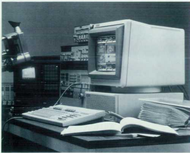
Fig. 1. Sophisticated instrumentation solutions are possible with a Series 300 Computer interfaced to the instruments using the HP-UX 5.0 device I/O library.
